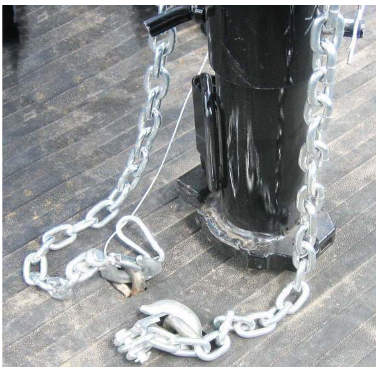
Safety Chain and Breakaway Brake Attachment Gooseneck
