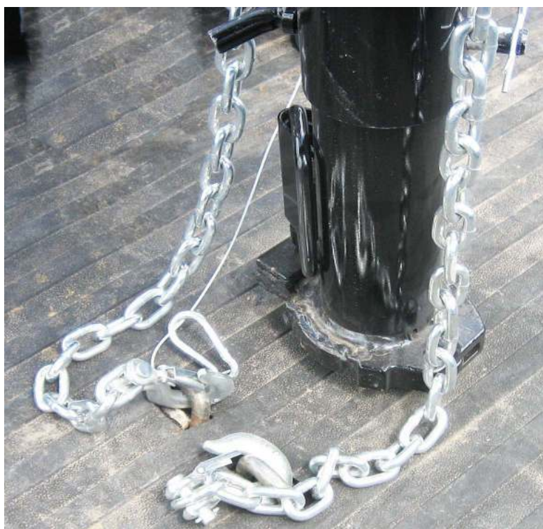
Safety Chain and Breakaway Brake Attachment Gooseneck
